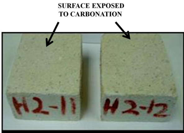
FIGURE 1. Concrete specimens measuring 15×15×7.5 cm 3 .
