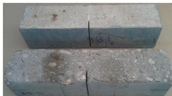
FIGURE 3. Samples subjected to 28 freeze-thaw cycles already notched. SFC front, AEAC rear.
