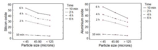
FIGURE 7. Particle size-activation time interaction graphs for SiO<sub>2</sub> and Al<sub>2</sub>O<sub>3</sub>. Chemical process at 80°C.
