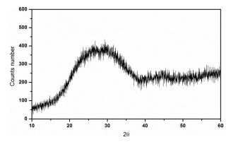
FIGURE 1. XRD diffractogram for the waste glass.
