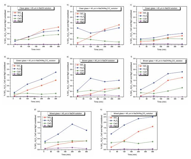
FIGURE 4. Chemical process at ambient T. Solubility of Si, Al, Ca and Mg oxides present in the four types of glass in alkaline media (NaOH and NaOH/Na<sub>2</sub>CO<sub>3</sub>).
