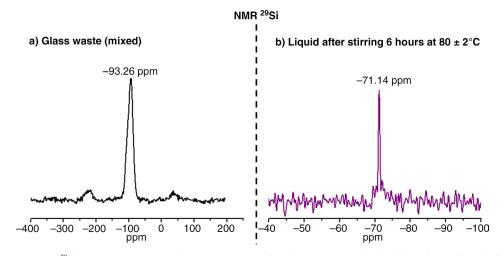
FIGURE 10. <sup>29</sup>Si MAS NMR spectra for a) untreated solid glass waste; and b) liquid obtained after stirring waste in a NaOH/Na<sub>2</sub>CO<sub>3</sub> solution for 6 hours at 80 ± 2 °C.
