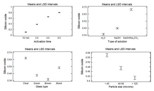
FIGURE 5. Significant main factors for SiO<sub>2</sub> solubility in chemical process at ambient temperature.
