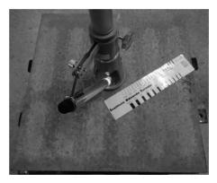
FIGURE 4. Crack width determined by mean of magnifying glass.
