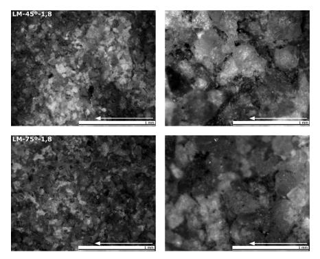
FIGURE 7. Detail of the tests after cleaning with 1.8mm nozzle on the toothed chisel valley — arrow: blasting direction —. USB digital microscope image.
