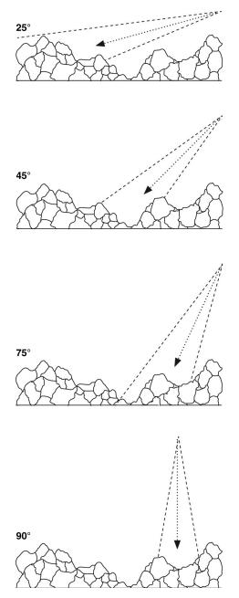
FIGURE 5. Blasting scheme on the surface with the different angles used in the trials.
