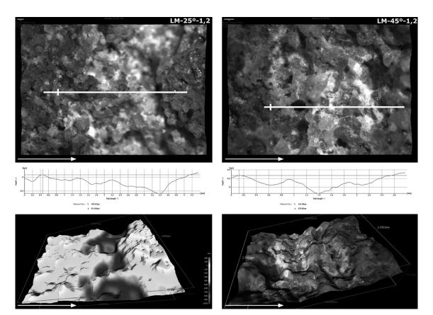
FIGURE 3. Detail of the topography and primary profile after cleaning with 25° and 45° on the toothed chisel valley — arrow: blasting direction —. Stereomicroscope with 3D visualizing and measuring image. Scale 200 μm.
