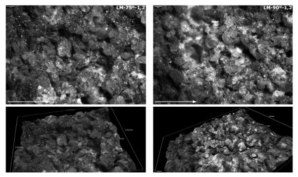
FIGURE 4. Detail of the topography after cleaning with 75° and 90° on the toothed chisel valley — arrow: blasting direction —. Stereomicroscope with 3D visualizing and measuring image. Scale 200 µm.
