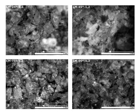
FIGURE 2. Detail of the tests after cleaning with 1.2 mm nozzle on the toothed chisel valley — arrow: blasting direction —. USB digital microscope image.
