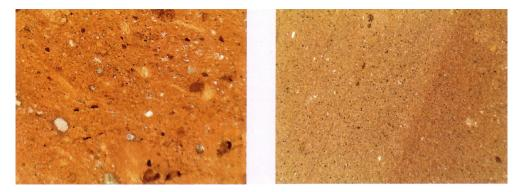
FIGURE 2. On the left a section of a brick tiles and right section of a modern brick made with microscope with 100x magnification.
