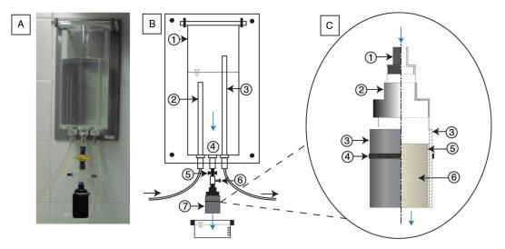
FIGURE 3. Constant head permeameter: (A). Constant head apparatus. (B). Schematic diagram: 1. Tank with over flow. 2. Inflow water. 3. Outflow water. 4. Water exit to the sample. 5. Valve to fit the sample. 6. Valve to purge the sample. 7. Sample. (C). Sample preparation: 1. PVC connection cup. 2. PVC screw fitting. 3. Heat shrinkable sleeve. 4. Adjusting flange. 5. PTFE. 6. Sample.
