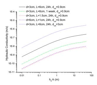
FIGURE 6. Hydraulic conductivity abacuses for the falling head method. Experimental parameters: height and diameter, d<sub>col</sub>, of the water column, testing time and size (diameter, d, and length, L) of the sample for the height variation from initial head, h0, to final head, h.
