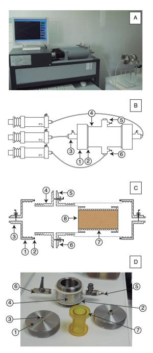
FIGURE 2. Triaxial method. Schematic diagram of triaxial cell.
