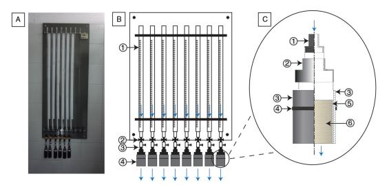
FIGURE 4. Falling head permeameter (8 tubes). (A). Falling head apparatus (8 tubes). (B). Schematic diagram: 1. Crystal tube.
