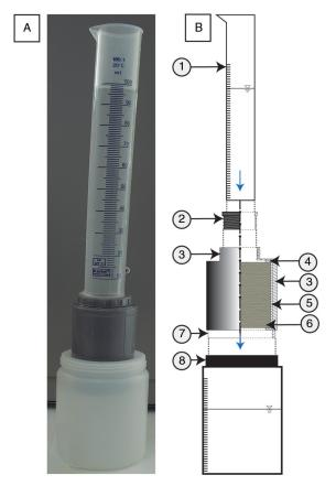
FIGURE 5. Falling head permeameter (Single graduated cylinder). (A). Falling head apparatus. (B). Schematic diagram: 1. Graduated cylinder. 2. PVC screw fitting. 3. PVC cell to house the sample. 4. Rubber joint. 5. PTFE. 6. Sample. 7. End piece to fit the PVC cell into the container. 8. Container to collect the water.
