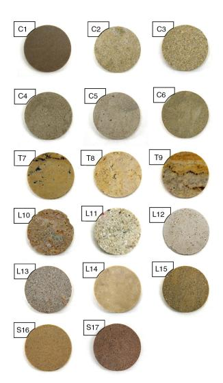
FIGURE 1. Image of the studied samples. C: biocalcarenites. T: travertines. L: allochem limestones. S: silica cement sandstones.
