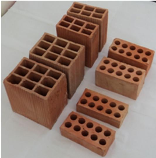
FIGURE 3. Examples of factory-scale produced sedimentary clay bricks.
