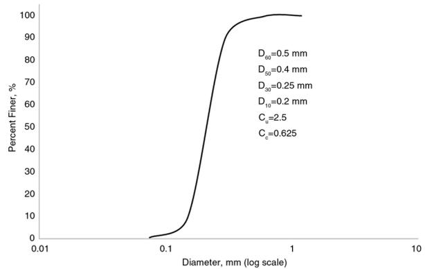
FIGURE 1. Grain size distribution curve for sand admixture.
