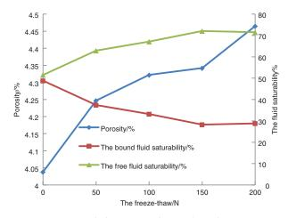
FIGURE 5. Variation curves of natural pumice concrete porosity and fluid saturation with respect to the number of freeze-thaw cycles (*N*).
