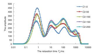
FIGURE 7. The distribution of the  $T_2$  spectrum of natural pumice concrete for different numbers of freeze-thaw cycles (N).
