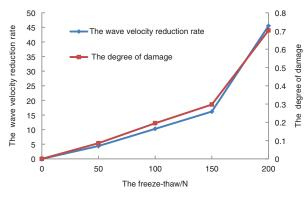
FIGURE 4. The variation curves of the wave velocity reduction rate and degree of damage with respect to the number of freeze-thaw cycles (*N*) of the lightweight aggregate concrete.
