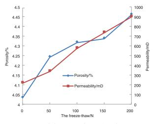
FIGURE 6. Variation curves of natural pumice concrete porosity and permeability with respect to the number of freeze-thaw cycles (N).
