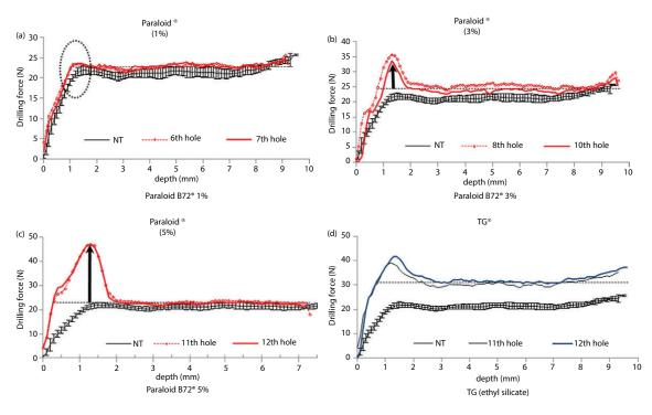
FIGURE 4. Drilling resistance curves for ceramic specimens treated with Paraloid B72® (a, b, c) and ethyl silicate (d).
