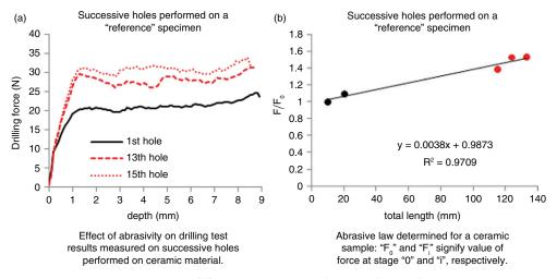
FIGURE 2. Drilling resistance on abrasive ceramic materials.
