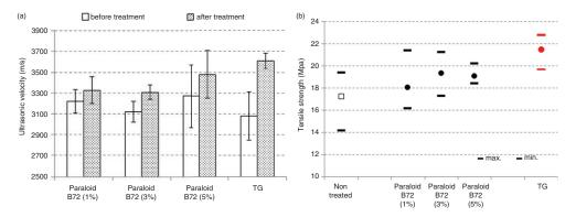
FIGURE 3. Ultrasonic velocity (on the left) and tensile strength (on the right) obtained on treated and non-treated ceramics consolidated with ethyl silicate (TG) and different formulation of Paraloid<sup>®</sup>
