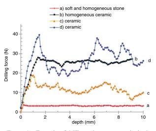
FIGURE 1. Examples of drilling resistance curves obtained on materials: a) soft and very homogeneous stone; b) homogeneous ceramic (used in this paper); c) and d) very heterogeneous old paving tiles with a superficial hard layer.
