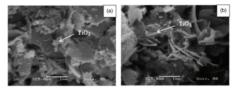
FIGURE 3. SEM micrographs of ZnAl-LDH/TiO<sub>2</sub> powders obtained only by mechanical activation (a. B1 - 3wt.% TiO<sub>2</sub>, b. B2 - 10wt.% TiO<sub>2</sub>).
