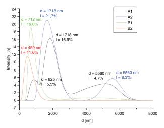
FIGURE 1. Particle size distribution of the ZnAl-LDH/ TiO<sub>2</sub> powders impregnated by vacuum evaporation prior to the mechanically activation (A1 – 3wt.% TiO<sub>2</sub>, A2 – 10wt.% TiO<sub>2</sub>) and only mechanically activated (B1 - 3wt.% TiO<sub>2</sub>, B2 – 10wt.% TiO<sub>2</sub>).
