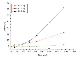
FIGURE 6. Photocatalytic activity of the coatings formed with 0.1g A2 /B2 powder and 0.5g B2 powder.
