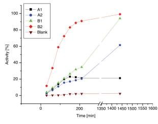
FIGURE 5. Photocatalytic activity of A1, A2, B1 and B2 powder samples and of the blank sample of RhB solution.
