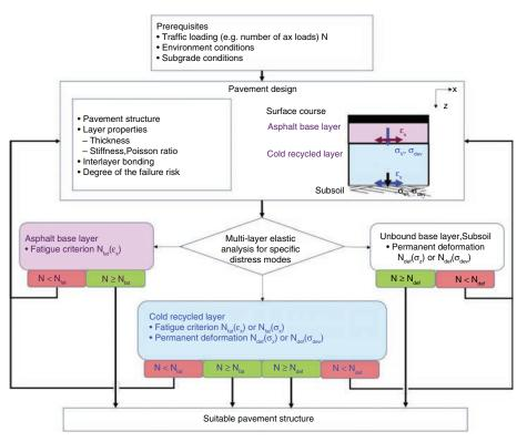
FIGURE 1. Analytical design principle for pavements with cold recycled layer (22).
