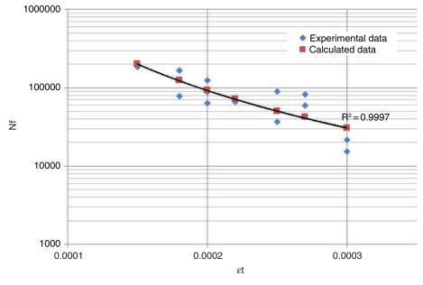
FIGURE 4. CRBM fatigue law calculation.
