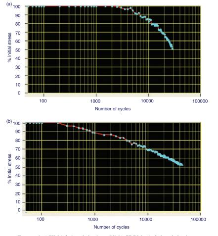
FIGURE 6. a) HMA fatigue behaviour (38) b) CRBM mix fatigue behaviour.
