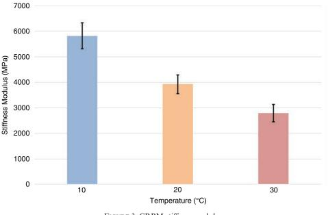
FIGURE 3. CRBM stiffness modulus.
