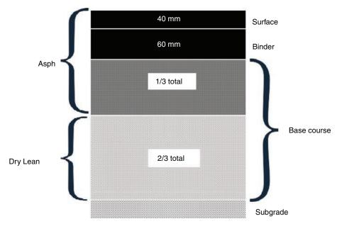
FIGURE 2. Airfield flexible pavement structure.
