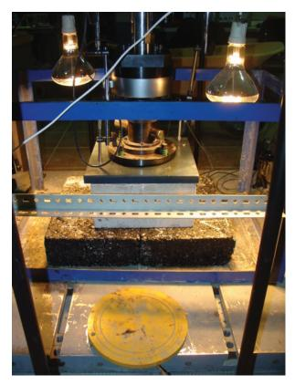
FIGURE 3. Plate bearing test and pressure cell.
