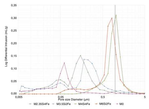
FIGURE 4. Differential mercury intrusion porosimetry (MIP) at 28 days.
