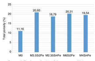
FIGURE 5. Total porosity (%) of the mortars at 28 days.
