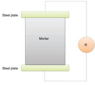
FIGURE 1. Two-electrode testing on mortar prism.
