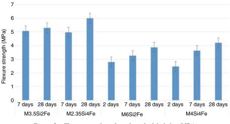
FIGURE 2. Flexure strength results and standard deviation (MPa).
