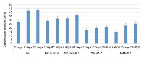
FIGURE 3. Compressive strength results and standard deviation (MPa).
