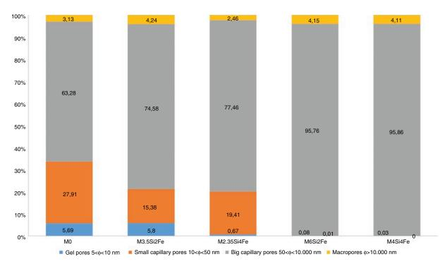
FIGURE 6. Pore-size distribution (PSD) of the mortars at 28 days.
