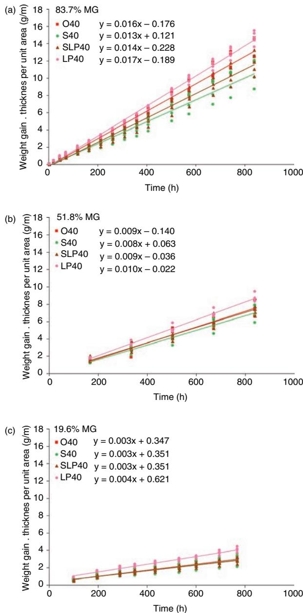
FIG. 4. WVT· $\Delta x$  in concrete mixes with different SCMs and w/cm = 0.40, MG = (a) 83.7%, (b) 51.8%, (c) 19.6%.
