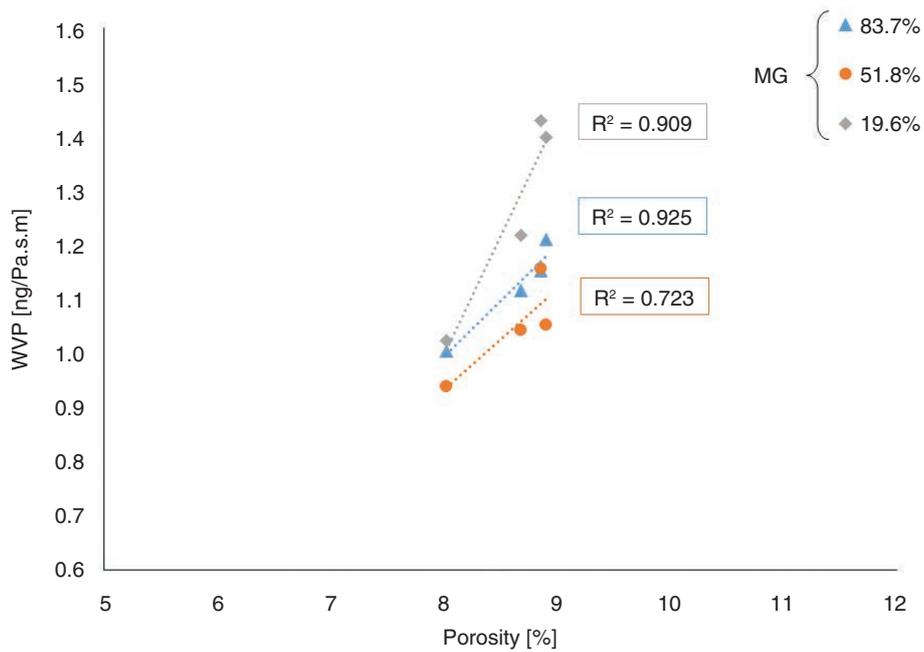
FIG. 6. Relationship between WVP and porosity of pure OPC concrete mixes for the different w/cm and MGs studied
