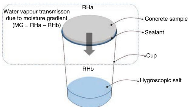
FIG. 1. Scheme of the set-up of the cup method.
