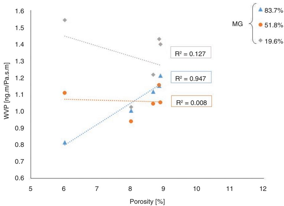
FIG. 7. Relationship between WVP and capillary porosity of pure OPC concrete mixes for the different w/cm and MGs studied
