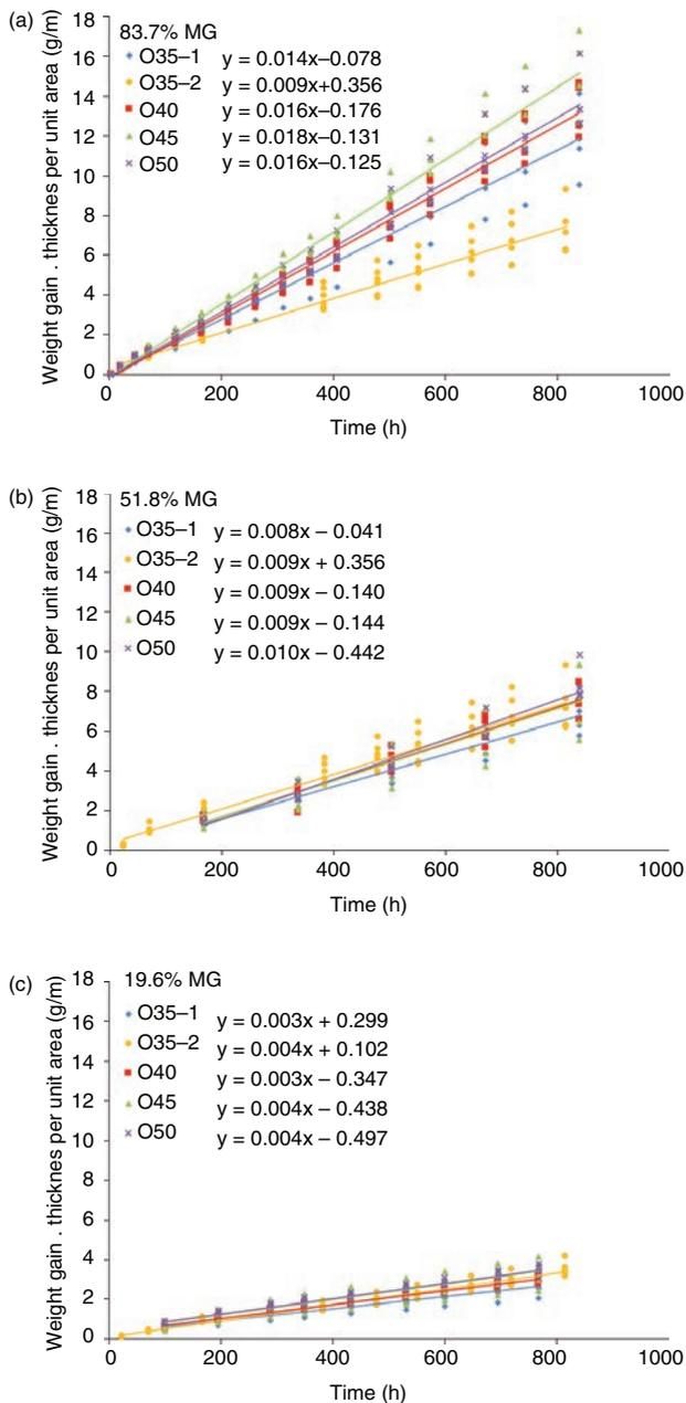
FIG. 3.  $WVT \cdot \Delta x$  in OPC concrete mixes with different w/cm, MG = (a) 83.7%, (b) 51.8%, (c) 19.6%.
