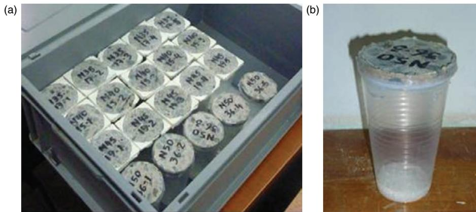
FIG. 2. Samples during the test (a), hygroscopic salt inside a cup where the concrete sample is the barrier (b)
