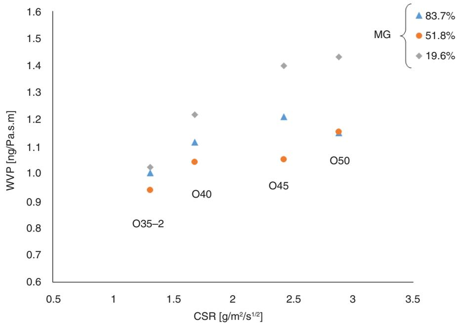
FIG. 9. Relationship between WVP and CSR of pure OPC concrete mixes for the different w/cm and MGs studied
