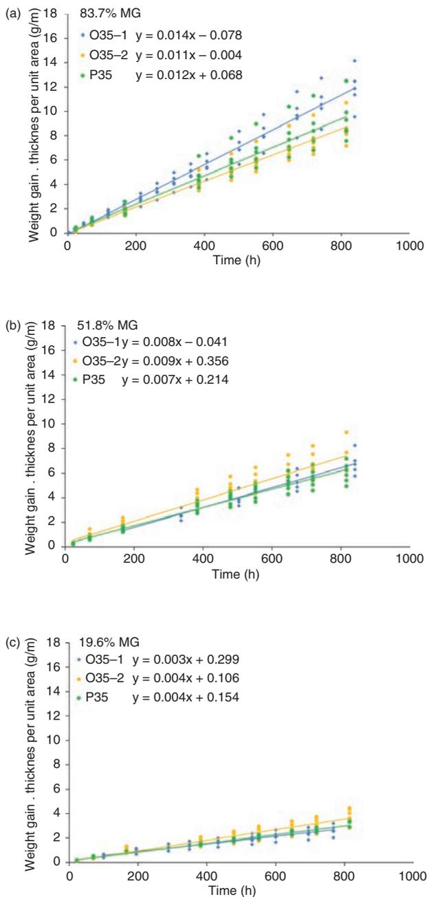
FIG. 5. WVT· $\Delta x$  in concrete mixes with  $w/cm = 0.35$ , MG = (a) 83.7%, (b) 51.8%, (c) 19.6%.
