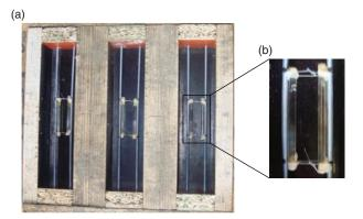
FIGURE 1. (a) Mold preparation for mortar prisms with self-healing properties; (b) Detail of the polyurethane filled capsules glued on nylon threads between the reinforcement bars
