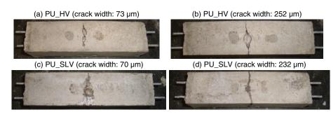
FIGURE 3. Crack healing of (a) a specimen with a relatively small crack width (< 100  $\mu$ m) healed by PU\_HV, (b) a specimen with a relatively large crack width (> 200  $\mu$ m) healed by PU\_HV, (c) a specimen with a relatively small crack width (< 100  $\mu$ m) healed by PU\_SLV and (d) a specimen with a relatively large crack width (> 200  $\mu$ m) healed by PU\_SLV
