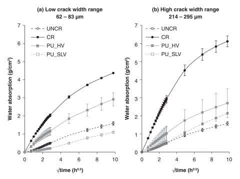
FIGURE 5. Cumulative water absorption curves in function of the square root of time for (a) specimens in the 'low crack width range' and (b) specimens in the 'high crack width range'. Error bars represent the standard error on the mean values
