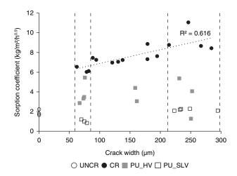
FIGURE 4. Capillary sorption coefficient in function of crack width for uncracked specimens, cracked specimens and specimens healed by PU\_HV or PU\_SLV. The dotted line represents the linear trend line that was fitted to the data of the cracked specimens. The vertical dashed lines represent the limits for the 'low' and 'high' crack width ranges
