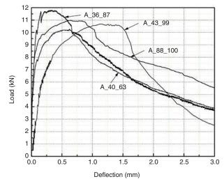
FIGURE 7. Load-deflection curves of beams with various sand graduations.
