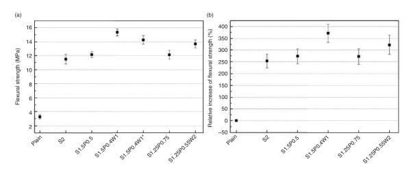
FIGURE 10. Properties of slab with different sand gradations (a) Flexural strength and (b) Relative increase of flexural strength.
