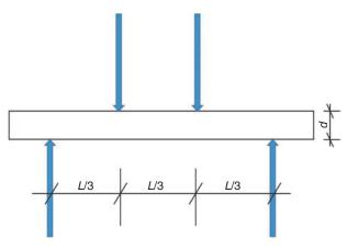
FIGURE 3. Schematic diagram of specimen under four-point flexural test.
