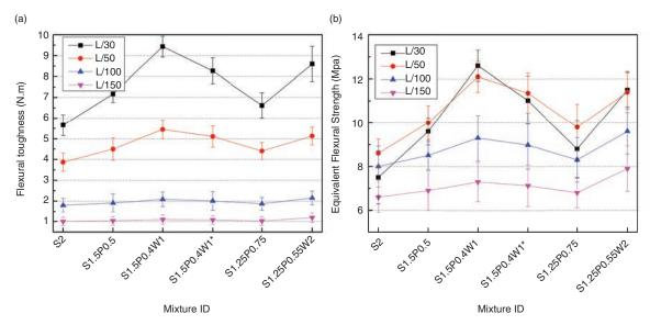
FIGURE 12. Flexural properties with different fiber combinations (a) Flexural toughness and (b) Equivalent flexural strength of composites up to specific deflection.
