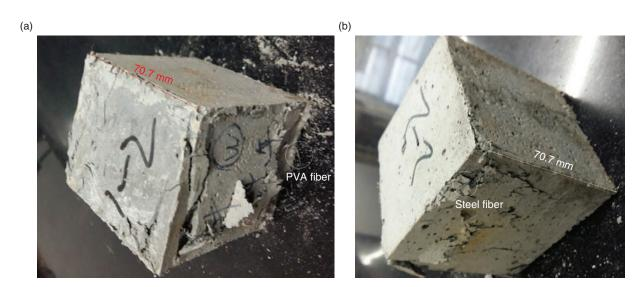
FIGURE 5. Typical fracture morphology of cubes after compressive strength test with different sand gradation (a) A\_40\_63 and (b) A\_36\_87.
