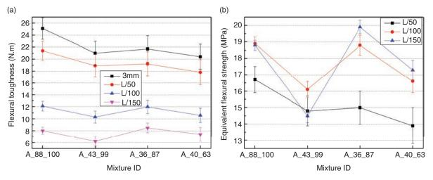
FIGURE 8. Properties of beam with different sand gradation (a) Flexural toughness and (b) Equivalent flexural strength of composites up to a specific deflection.
