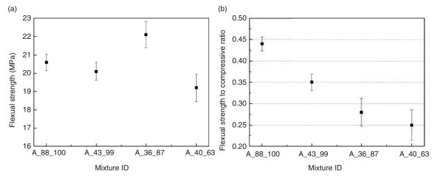
FIGURE 6. Properties of beams with different sand gradations (a) Flexural strength and (b) Flexural strength to compressive strength ratio.
