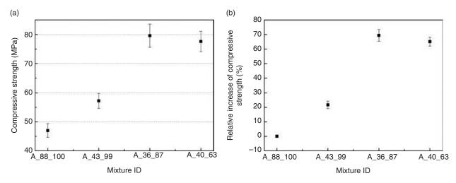
FIGURE 4. Properties of cubes with different sand gradations (a) Compressive strength and (b) Relative increase of compressive strength.
