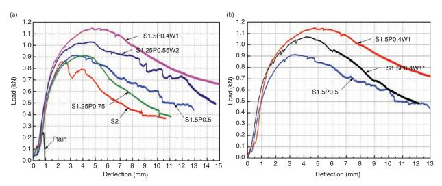
FIGURE 11. Load-deflection curves of slab with various parameters (a) different fiber combination and (b) various sizes of sand.
