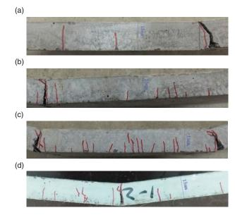
FIGURE 13. Typical failure pattern of slab after flexural testing with different fiber combinations (a) S2 (b) S1.5P0.5 (c) S1.5P0.4W1 (d) S1.5P0.4W1\*.
