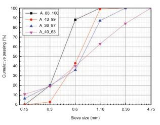
FIGURE 1. Sieve analysis of different types of sands.
