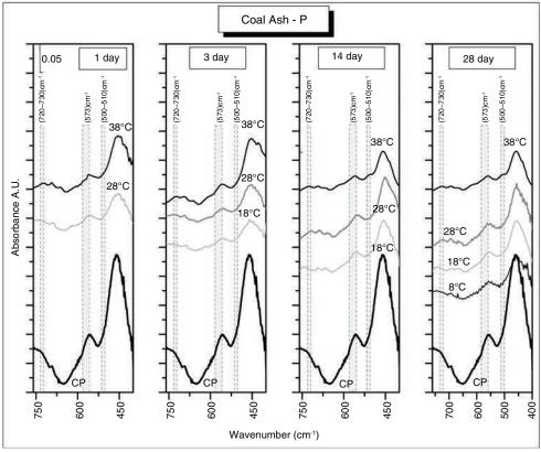
FIGURE 7. FTIR spectra in zone 2 for both ashes and their activation products at different temperatures and curing ages
