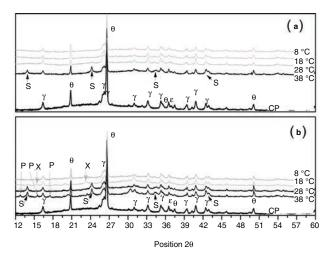
FIGURE 2. Diffractograms of the CP ash (a) 3 days and (b) 28 days of curing. θ: Quartz, γ: Mullite, ε: Hematite, S: Sodalite, P: Zeolite Phi, X: Zeolite X.
