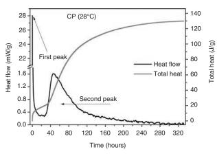
FIGURE 8. Microcalorimetry at 28 °C for CP ash
