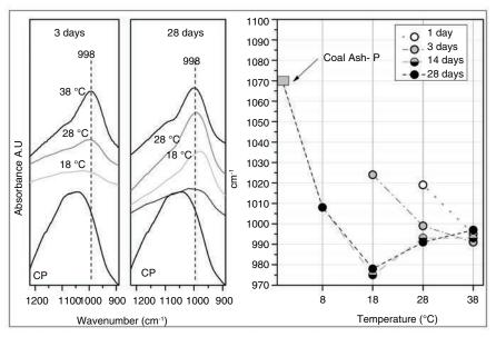
FIGURE 6. Displacement of the band between 1100 cm<sup>-1</sup> and 970 cm<sup>-1</sup> of the FTIR depending on temperature and time for study ashes
