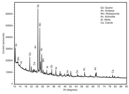
FIGURE 2. X-ray diffraction of fine concrete waste. Where Qz is quartz, An is anatase, Wn is wollastonite, Ac is actinolita, Al is albite and Ca is calcite. (Mejia et al. (29) source).
