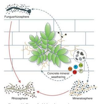
FIGURE 10. Draw of a higher plant growing on a concrete material. The plant roots exudate carbonaceous compounds that promote growth of microbial population in the mineral matrix; this is an equivalent concept to the mineralsphere proposed by Uroz et al. (34) in plant-soil systems.
