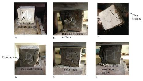
FIGURE 6. Fractured surfaces, a. Plain mortar, b. 2% Rice straw reinforced mortar, c. 2% Sisal fibre reinforced mortar, d. 5% Rice straw reinforced mortar, e. 5% Sisal fibre reinforced mortar, and f. 2% Treated rice straw reinforced mortar.
