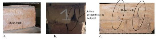
FIGURE 9. Fractured surfaces in blocks: a. Single block, b. 1x2 blocks, and c. 2x2 blocks.
