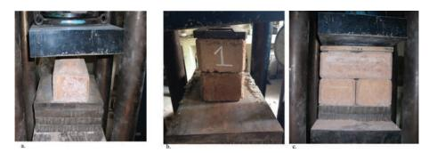
FIGURE 4. Test set up of ISSBs, a. Single block, b. 1x2 blocks, and c. 2x2 blocks.
