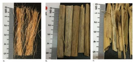
FIGURE 2. Fibres used, a. Sisal, b. Rice straw, and c. Treated rice straw.
