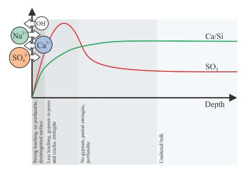
FIGURE 1. Schematic profile of ESA by sodium sulfate solution (adapted from Ref. 25).
