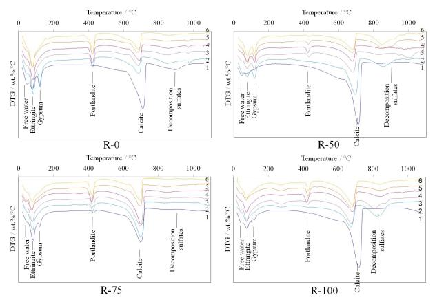
FIGURE 6. DTG patterns for samples at different depths of concretes.
