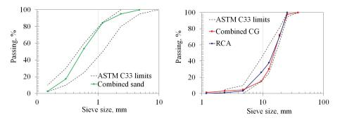
FIGURE 2. Particle size distribution of aggregates.
