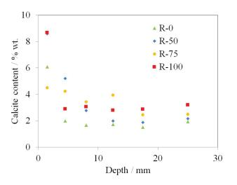
FIGURE 7. Calcite profiles computed from TG/DTA.
