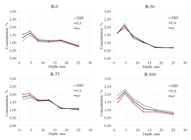
FIGURE 5. Sulfate profiles of RACs determined by CA and XRF.
