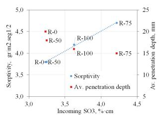
FIGURE 8. Incoming SO<sub>3</sub> and transport properties.
