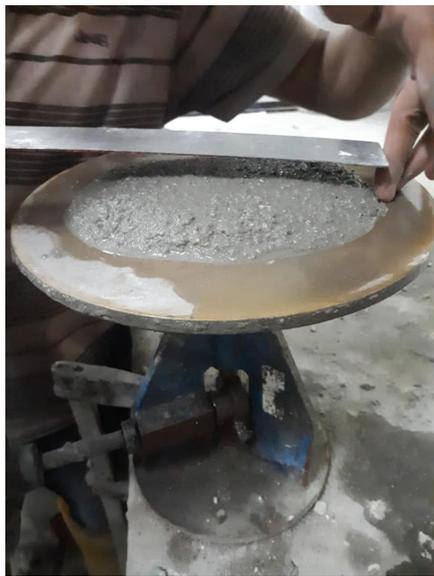
FIGURE 2. The flow table test.
