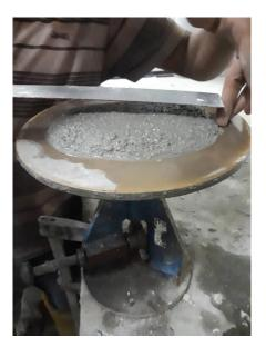
FIGURE 2. The flow table test.
