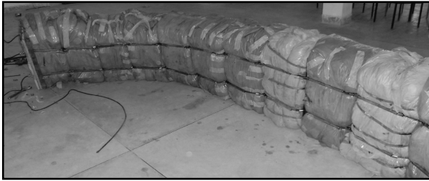
Figure 10. The arch gradually curving by pre-stressing.
