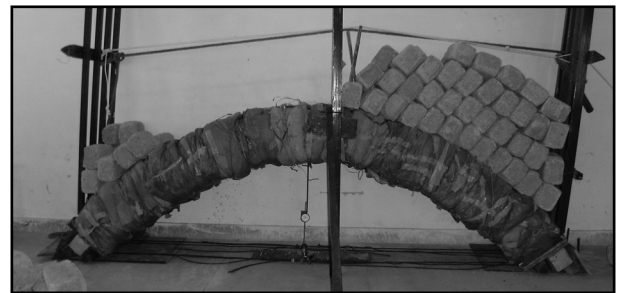
Figure 14 Arch subjected to unsymmetrical loading.
