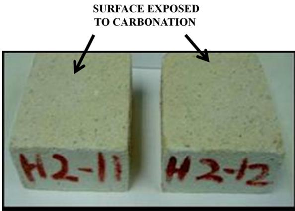
FIGURE 1. Concrete specimens measuring 15×15×7.5 cm<sup>3</sup>.
