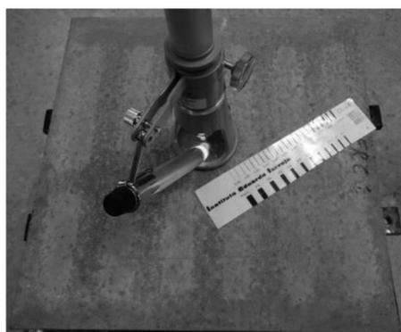
FIGURE 4. Crack width determined by mean of magnifying glass.
