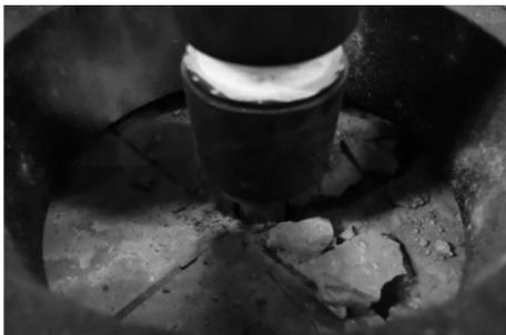
FIGURE 3. Finish of impact load test on a slab.
