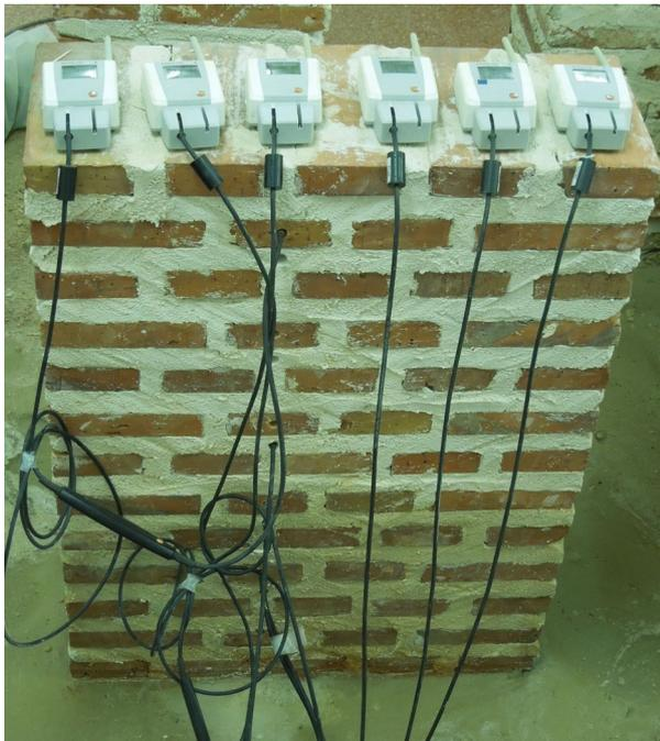
FIGURE 1. One foot brick tiles wall with moisture probes, standing on a bed of sand.
