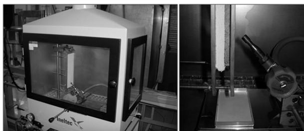
FIGURE 3. The left figure shows the apparatus used to determine sample flammability using the single flame test. The right figure shows the burner utilized in the test along with the vertically-placed test sample.
