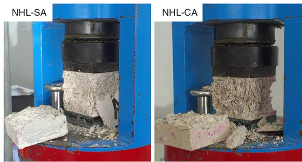
FIGURE 7. Appearance of mortars made with siliceous (NHL-SA) and calcareous (NHL-CA) sand and cured at a relative humidity of 90%, after the compressive rupture.
