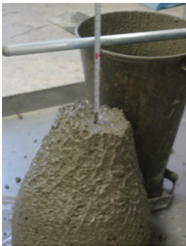
FIGURE 4. Aspect of the optimum mix using the sediment as substitution of fine aggregate.
