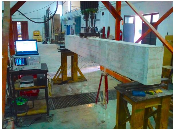
FIGURE 5. Experimental setup for the RC beams externally strengthened with CFRP.
