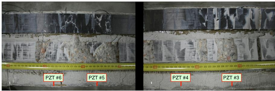
FIGURE 11. Damages with concrete cover separation between sensors 5 and 6 (left) and sensors 3 and 4 (right) for the RC-Beam #2.
