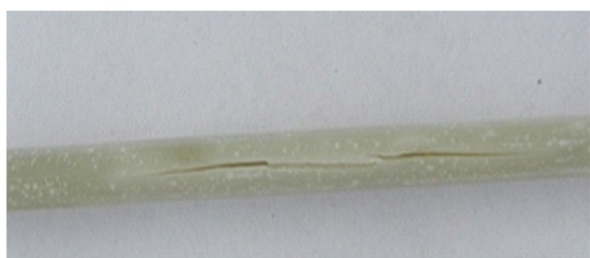
FIGURE 5. Longitudinal fissures in EC+25% TAC capsules due to storage in water for 7 days.
