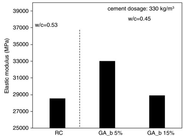
FIGURE 11. Young's modulus of GA concretes (w/c=0.45 and 330 kg/m<sup>3</sup> cement content) and reference mixture (w/c=0.53 and 330 kg/m<sup>3</sup> cement content).
