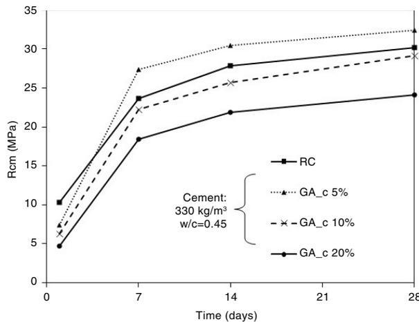
FIGURE 9. Compressive strength vs. age of GA concretes (w/c=0.45 and 350 kg/m<sup>3</sup> cement content) and reference mixture (w/c=0.53 and 330 kg/m<sup>3</sup> cement content).
