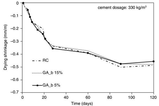
FIGURE 10. Drying shrinkage of GA concretes (w/c=0.45 and 330 kg/m<sup>3</sup> cement content) and reference mixture (w/c=0.53 and 330 kg/m<sup>3</sup> cement content).
