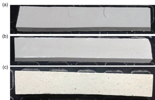
FIGURE 4. Appearance of the MK-based geopolymer composites after exposure to 1200 °C for 2 h: (a) G, (b) G-CF and (c) G-AFRP.
