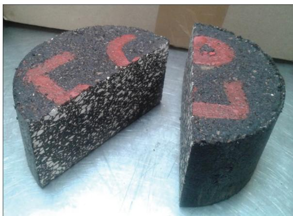
FIGURE 2. Marshall specimen of bituminous mortar split into two halves.
