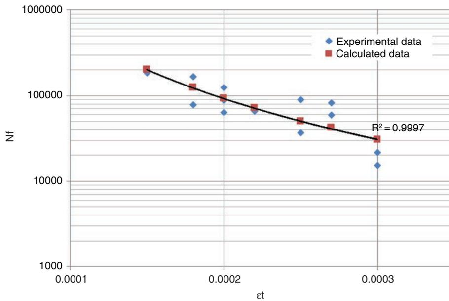
FIGURE 4. CRBM fatigue law calculation.
