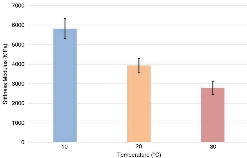
FIGURE 3. CRBM stiffness modulus.
