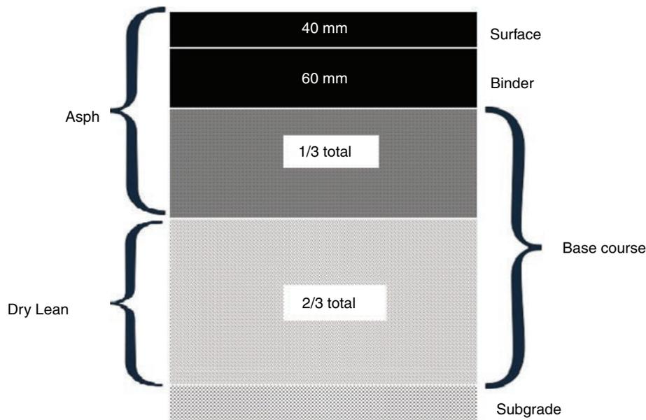
FIGURE 2. Airfield flexible pavement structure.
