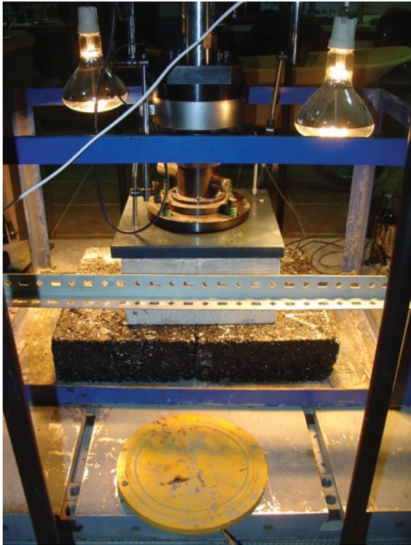
FIGURE 3. Plate bearing test and pressure cell.
