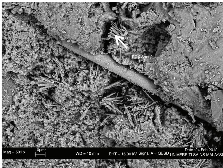
FIGURE 12. SEM image (501× magnification) of the 2.4 GF in the W-series at 18 months.
