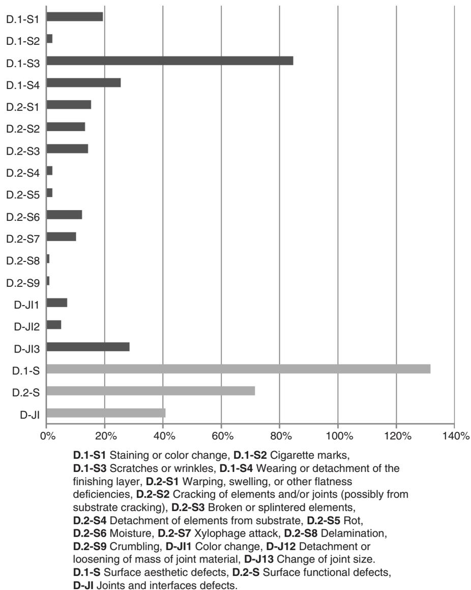
FIGURE 2. Relative frequency of the occurrence of defects and groups of defects in the 98 inspected wood floorings
