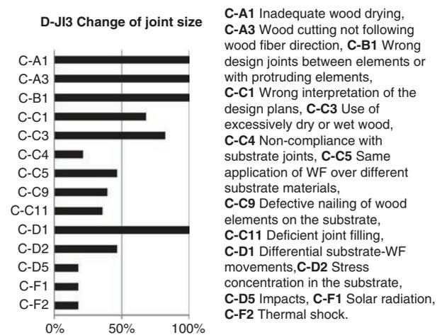
FIGURE 9. Contribution of probable causes to the 28 D-JI3 defects detected
