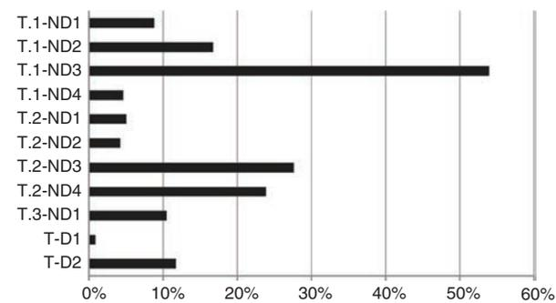
**T.1-ND1** Flatness evaluation, **T.1-ND2** Crack or fissure measurement, **T.1-ND3** Evaluation of other singularities, **T.1-ND4** Evaluation of biological actions, **T.2-ND1** Metal blade, **T.2-ND2** Percussion test, **T.2-ND3** Moisture measurement (surface and/or environmental), **T.2-ND4** Temperature measurement (surface and/or environmental), **T.3-ND1** Superficial hardness measurement, **T-D1** Pull-off test, **T-D2** Inner moisture measurement.
