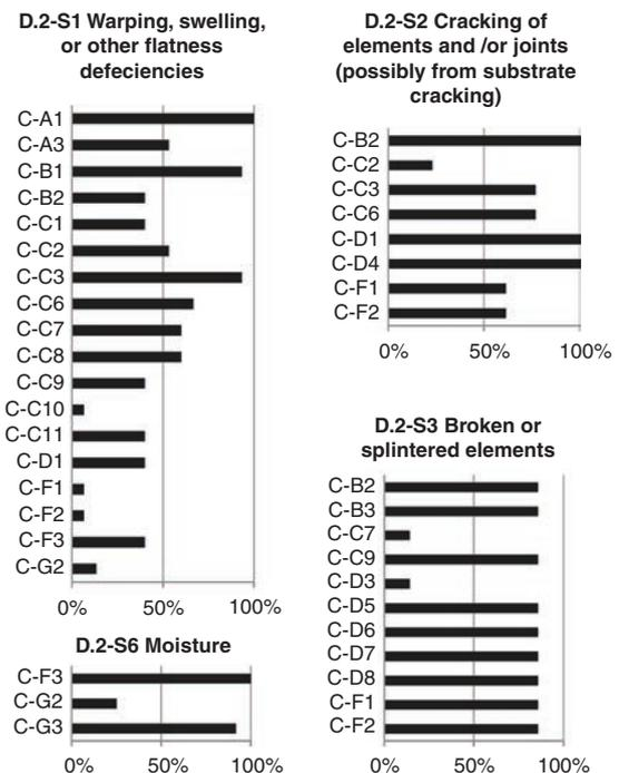
FIGURE 8. Contribution of probable causes to the most representative surface functional defects detected: D.2-S1 (15 detected defects), D.2-S2 (13 detected defects), D.2-S3 (14 detected defects) and D.2-S6 (12 detected defects)
