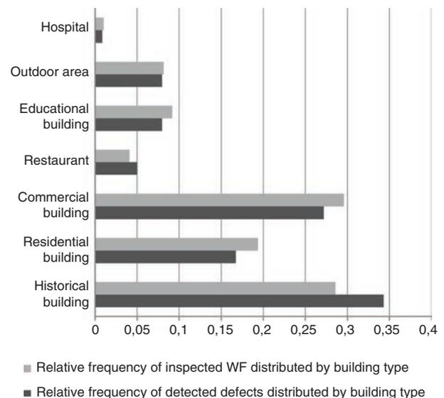
FIGURE 1. WF and detected defects distributed according to building type in the sample
