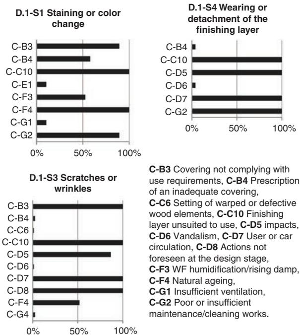
FIGURE 7. Contribution of probable causes to the most representative surface aesthetic defects detected: D.1-S1 (19 detected defects), D.1-S3 (83 detected defects) and D.1-S4 (25 detected defects)
