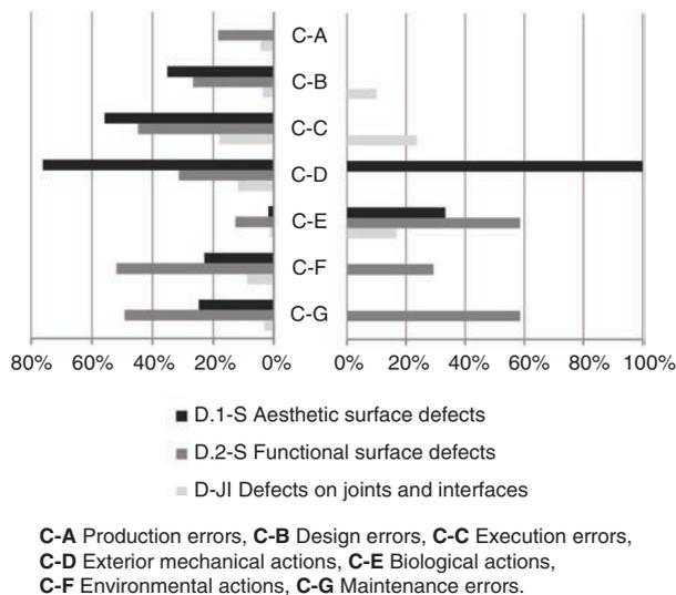
FIGURE 6. Relative frequency of the groups of probable causes, according to groups of defects they were attributed to, considering indirect causes on the left and direct causes on the right
