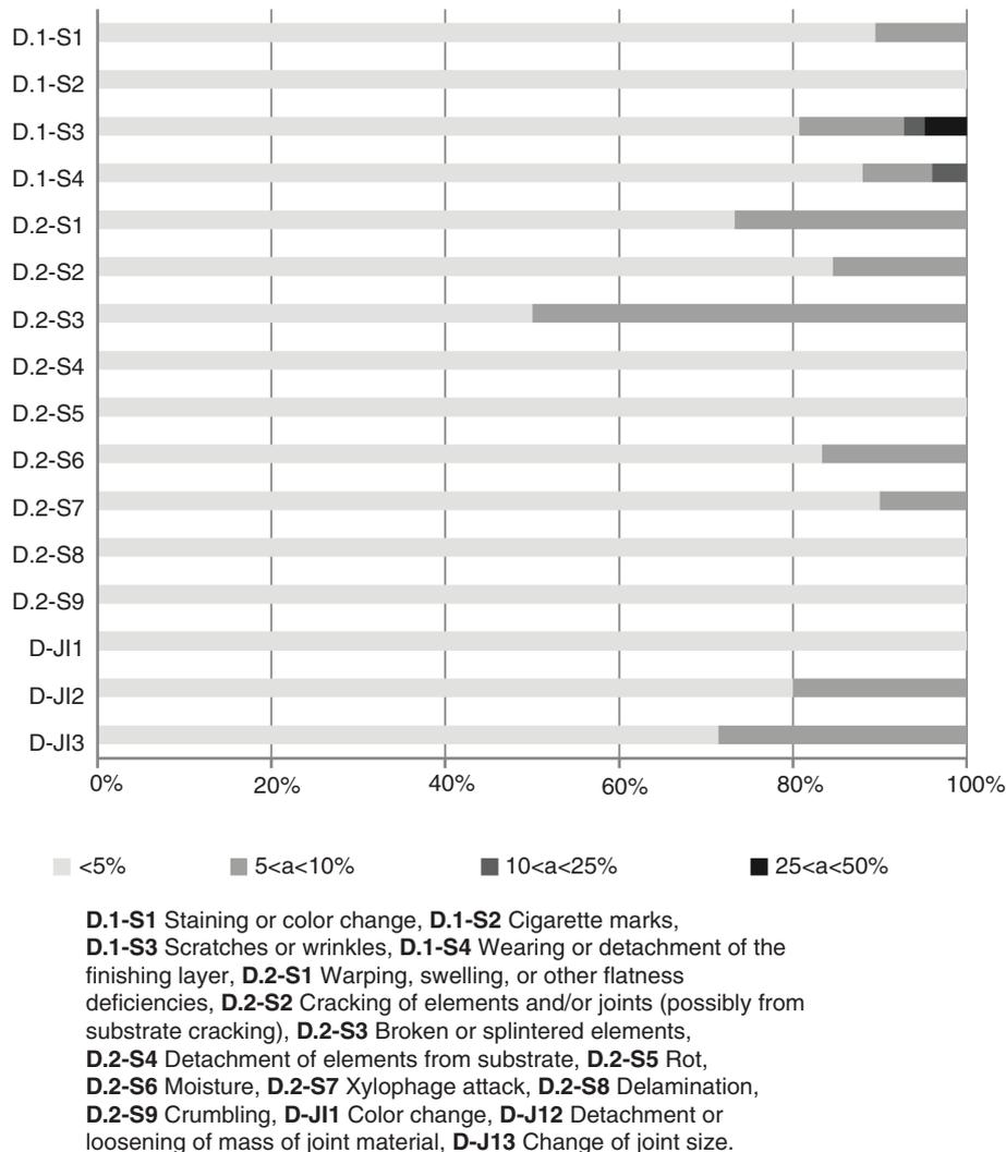
FIGURE 5. Relative frequency of the affected area per type of defect in the sample
