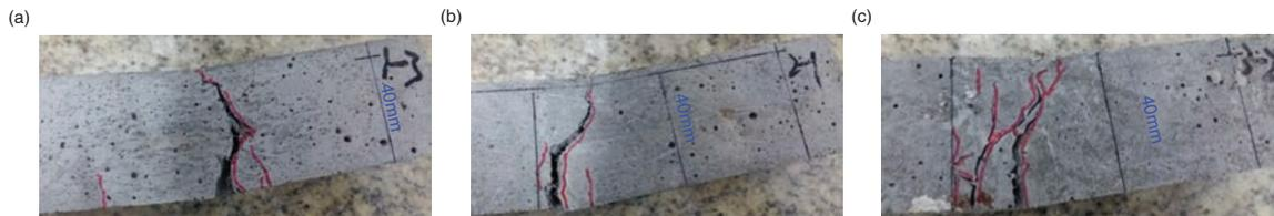
FIGURE 9. Typical failure pattern of beam after flexural strength test with different sand gradation (a) A\_40\_63, (b) A\_36\_87 and (c) A\_88\_100.
