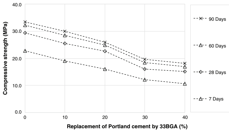
FIGURE 7. Relationship between the compressive strength of mortar and the replacement of Portland cement by 33BGA
