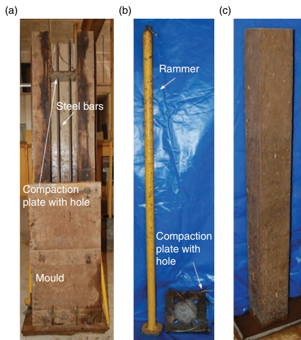
FIGURE 3. Details of equipment; (a) mould and reinforcement details; (b) rammer and compaction plate and (c) test specimen.
