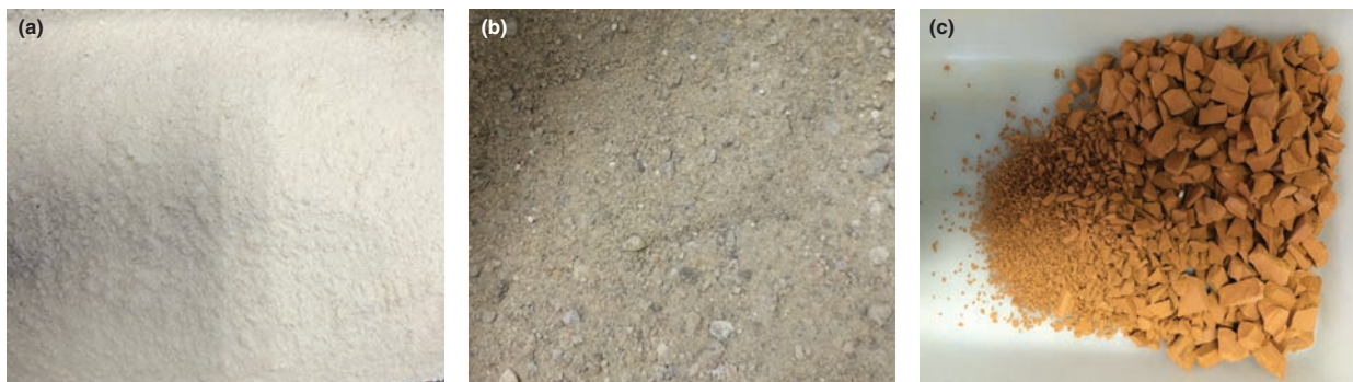
FIGURE 1. Materials before processing: Portland cement, natural aggregate, ceramic waste.
