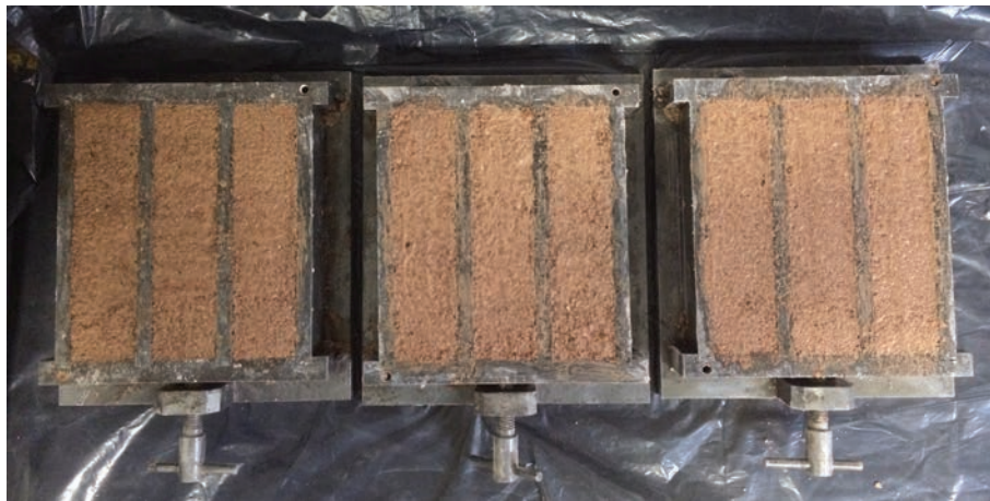
FIGURE 3. Manufacture of mortar specimens with 40% ceramic waste.
