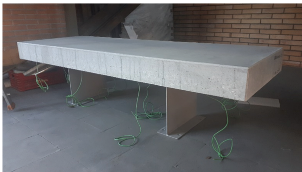
FIGURE 2. Visual aspect of the full-scale benches fabricated for the thermal characterization.
