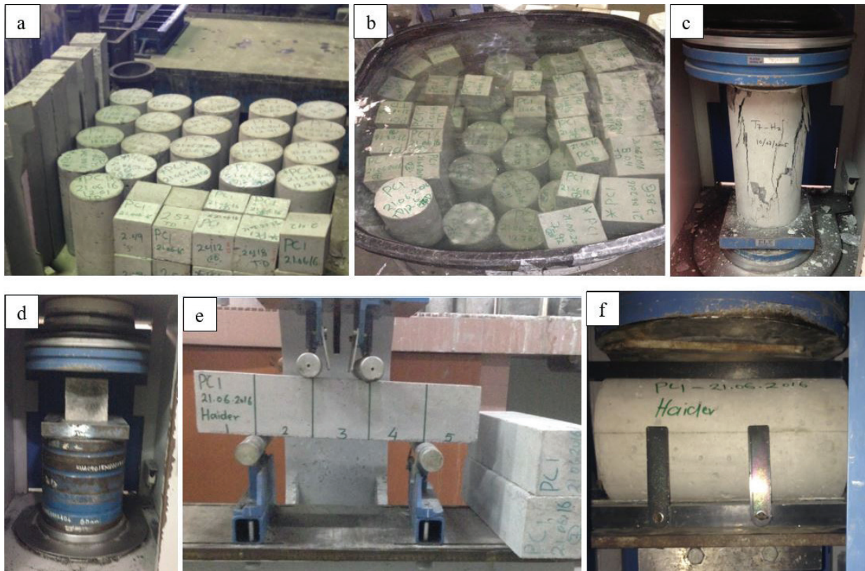
FIGURE 1. Experimental work of (a) concrete samples after de-moulding, (b) curing of samples, (c) and (d) compressive strength test, (e) flexural strength test, and (f) splitting-tensile strength test
