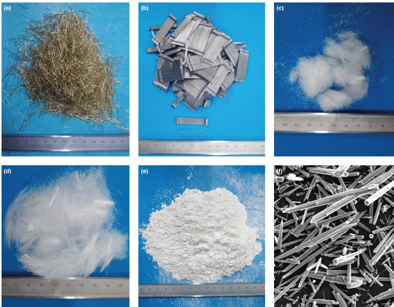
FIGURE 3. The fibers used in this study: Short steel fiber (SS); Long steel fiber (LS); Short PVA fiber (SP); Long PVA fiber (LP); \text{CaCO}_3 whisker (CW); SEM of CW.
