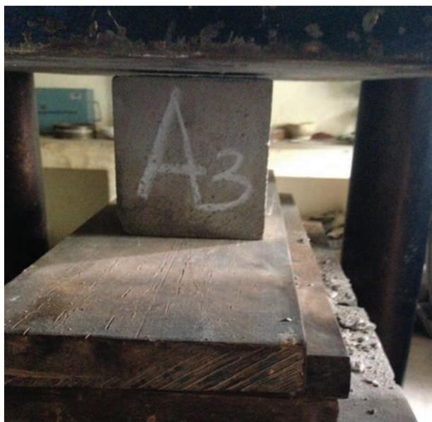
FIGURE 3. Typical test set up for mortar cubes.
