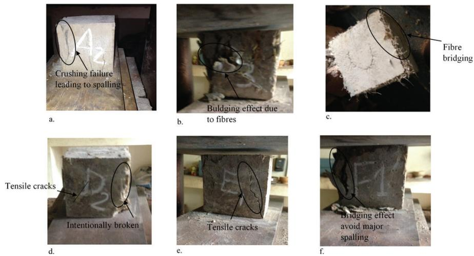
FIGURE 6. Fractured surfaces, a. Plain mortar, b. 2% Rice straw reinforced mortar, c. 2% Sisal fibre reinforced mortar, d. 5% Rice straw reinforced mortar, e. 5% Sisal fibre reinforced mortar, and f. 2% Treated rice straw reinforced mortar.
