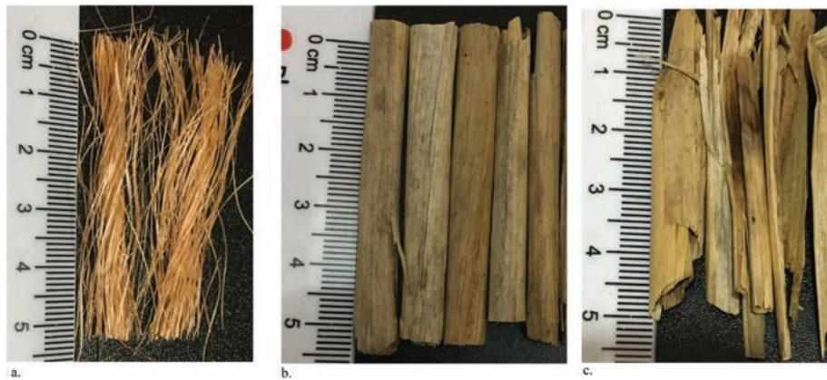
FIGURE 2. Fibres used, a. Sisal, b. Rice straw, and c. Treated rice straw.
