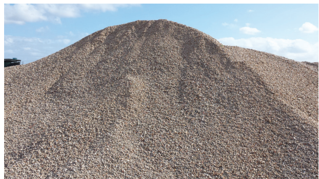
FIGURE 1. Pile of recycled aggregates in a recycling plant.
