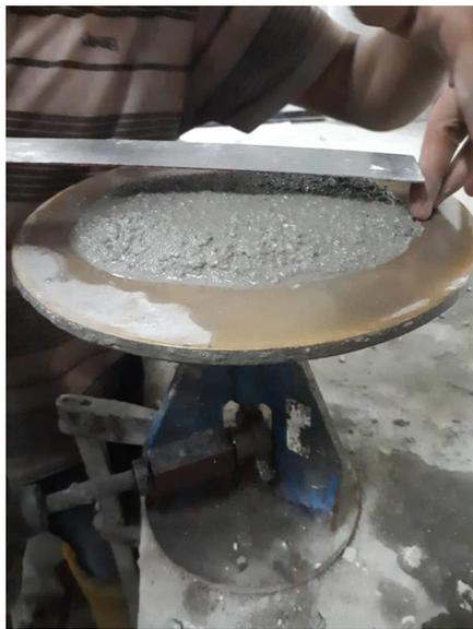
FIGURE 2. The flow table test.
