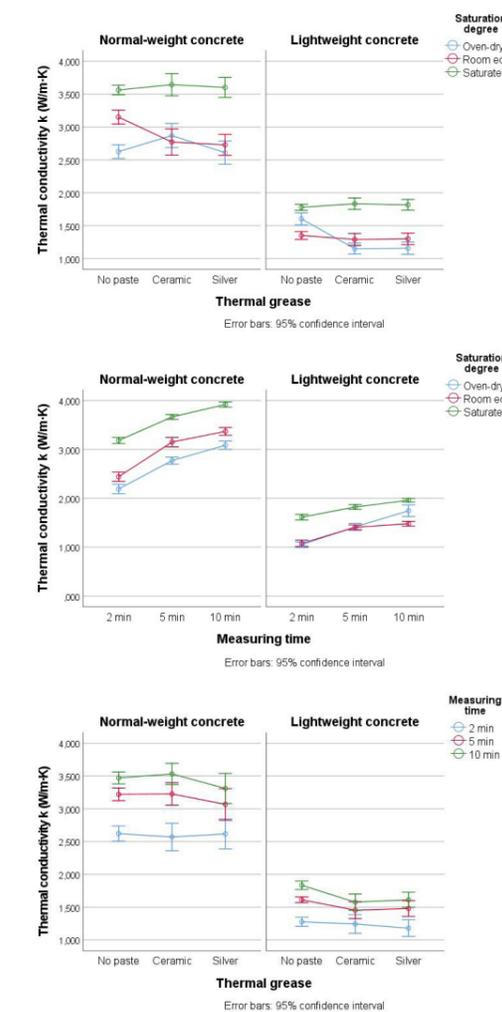
FIGURE 4. Graphs of the saturation degree\*thermal grease interaction (upper), saturation degree\*measuring time interaction (middle) and measuring time\*thermal grease interaction (lower) for normal-weight concrete and lightweight concrete.
