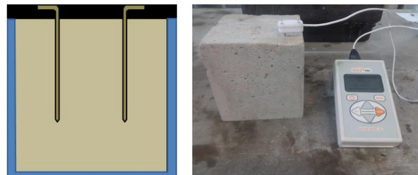
FIGURE 1. Left: Pilot-pin disposition during casting; Right: Measurement at room conditions.
