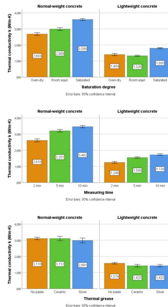
FIGURE 3. Overall means for the three main effects: saturation degree (upper), measuring time (middle) and thermal grease (lower), for normal-weight concrete and lightweight concrete.
