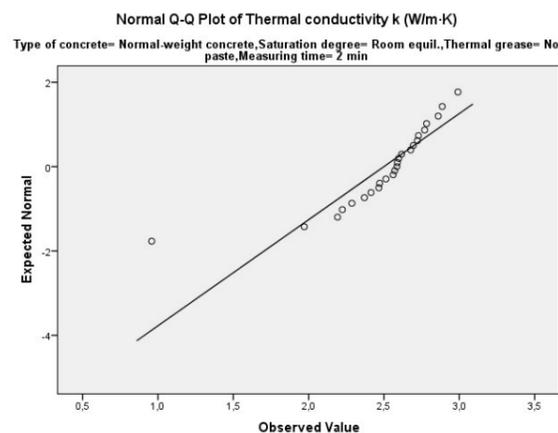
FIGURE 2. Q-Q plot of the 25 results for normal-weight concrete, concrete at equilibrium with the room conditions ( $T = 20 \pm 2^\circ\text{C}$ ,  $\text{RH} = 50 \pm 5\%$ ), no thermal grease applied within the measuring holes, measuring time = 2 min.
